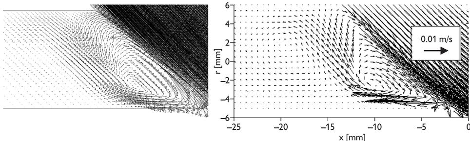
Figure 5 – Vortex structure in symmetry plane model in POS area with connection angle 45° and  $Re=1400$ . Left: numerical simulation, Right: PIV experimental measurement. A good quality and quantity agreement between numerical and experimental solution is visible.
