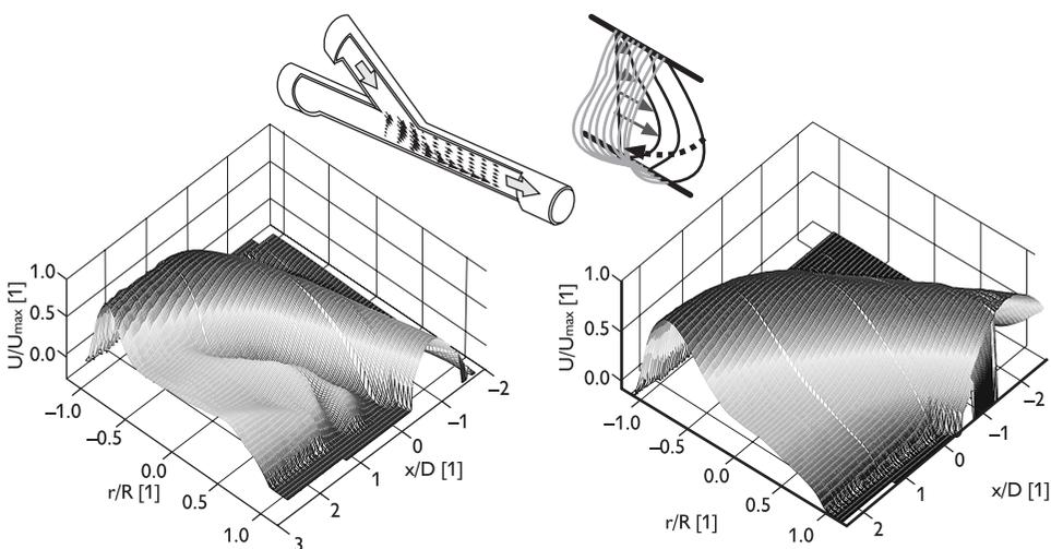
Figure 7 – Velocity distribution in  $x$  direction for  $Re$  1400 from PIV. Velocity in direction  $x$  is projected to the  $z$ -axis, as it is illustrated in the small pictures. Left: velocity fields in direction  $x$  for connection angle  $45^\circ$ . Right: velocity fields in direction  $x$  for connection angle  $20^\circ$ .
