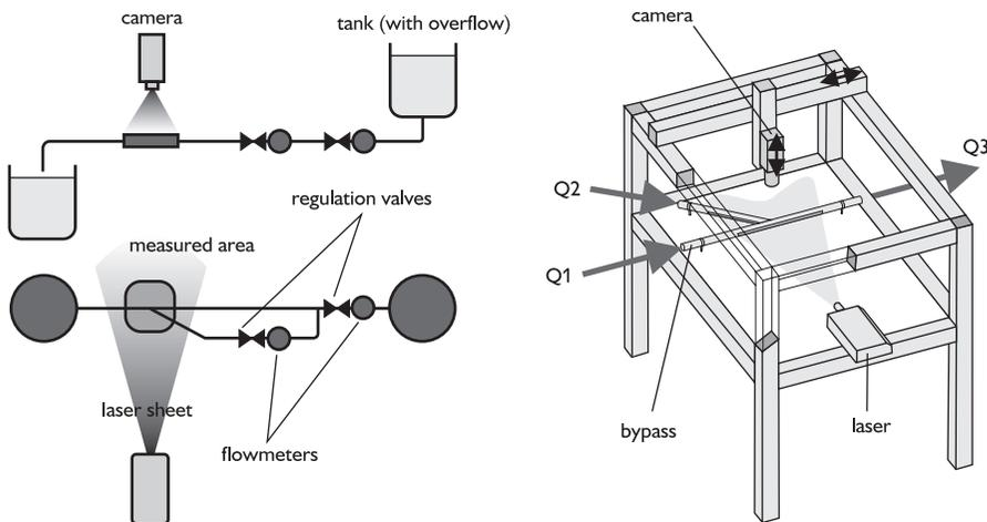
Figure 2 – Left: Experimental equipment for visualization and flow fields measurement by PIV. Right: Scheme of measuring place with fixed model.  $Q_1$ ,  $Q_2$ ,  $Q_3$  are flow rates in different parts of the model. Laser and camera are placed on the sliding equipments, which enabled illumination and taking photos of precisely determined place.
