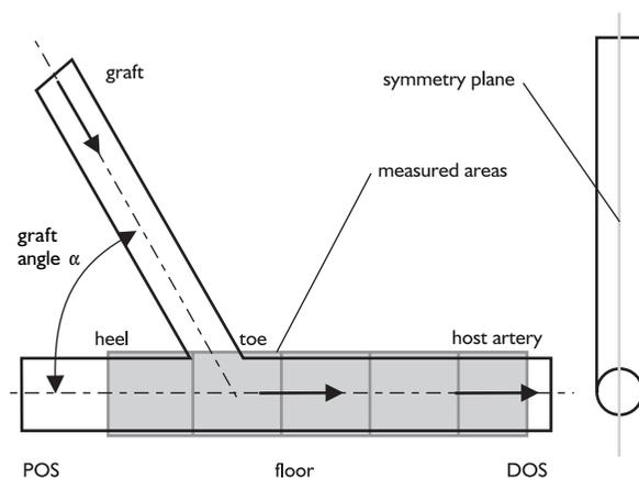
Figure 1 – Scheme of the bypass model for measurement by PIV method. In the picture the parts of bypass are illustrated: the symmetry plane where the PIV measurement was carried out, the measured areas, the areas of proximal outlet segment (POS) and distal outlet segment (DOS).
