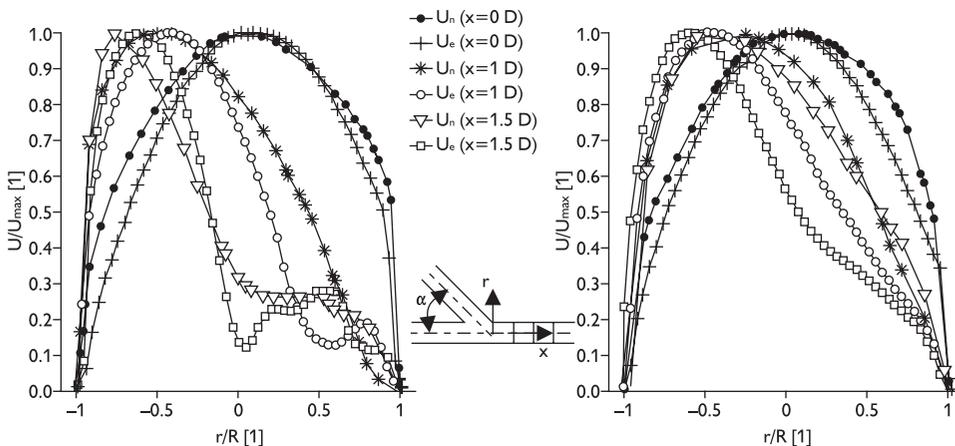
Figure 6 – Comparison of experimental (marked with subscript e) and numerical (marked with subscript n) velocity profiles in cross sections  $x = 0; 1; 1.5 D$ . Left: for angle  $\alpha = 45^\circ$ . Right: for angle  $\alpha = 20^\circ$ . In the pictures we can see a good agreement between numerical and experimental solution. Comparison of the flow fields shows that the region of secondary flow is bigger for angle connection  $\alpha = 45^\circ$ .
